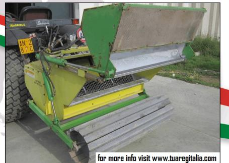
the depth adjustment is hydraulically controlled.
