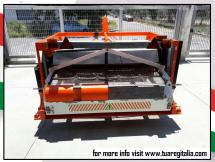
The Beach Cleaner works mechanically by taking the movement directly from the tractor's power takeoff, to which it is connected with the three-point linkage of the lift, which also adjusts the working depth from 0 to 15 cm for a width of 160 cm.
